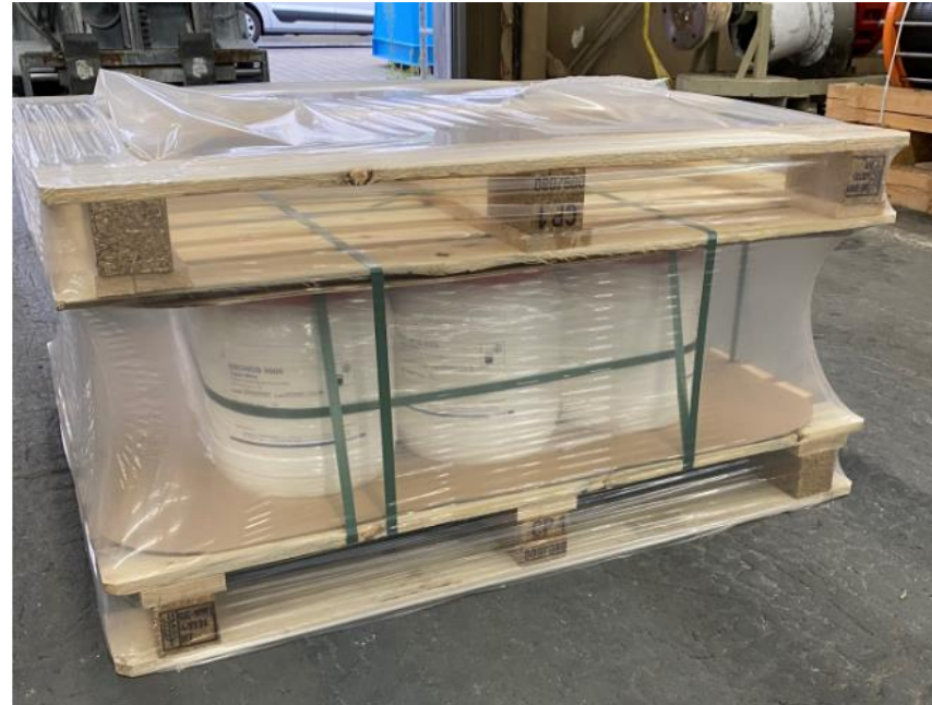
15L Drum (23 kg) -> single drum -> one palett: 9 x 15L
