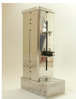
Trimaster - high speed filament stretching device which can be used for both extensional viscosity and filament break-up behaviour for low viscosity fluid.
