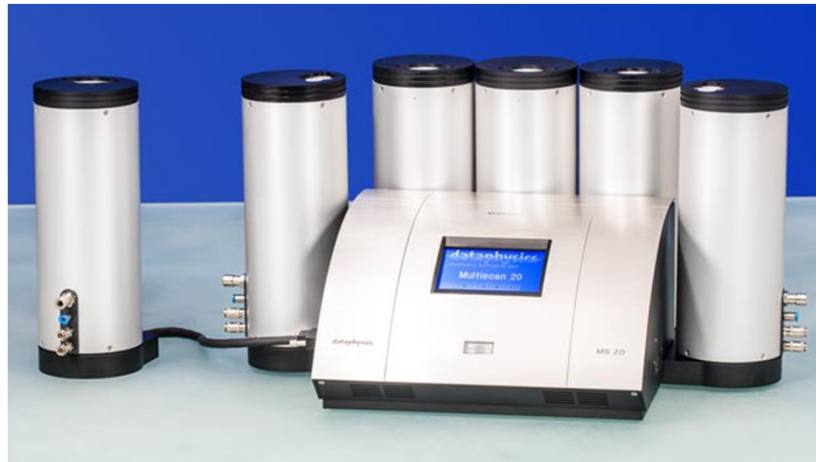
Optical stability analysis of liquid heterogeneous mixtures (suspensions, emulsions, foams)
